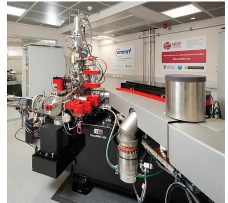
The labs at UWA pack superlative analytical power, including three CAMECA instruments. Above: the advanced NanoSIMS 50L ion microprobe.
